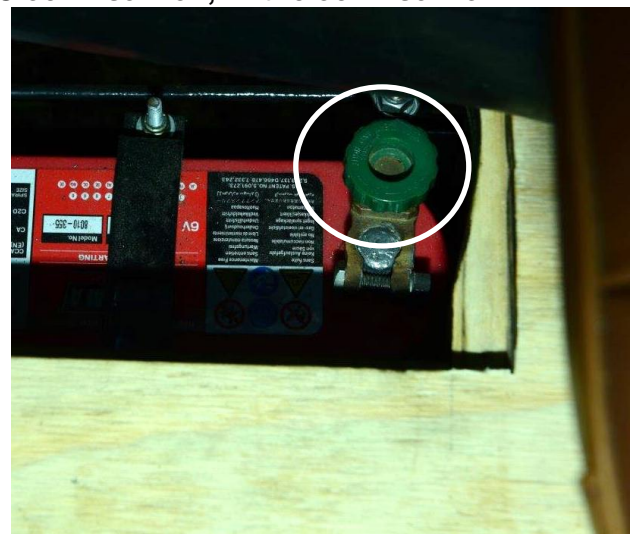
Location of Battery Switch (green) – Clockwise = on, Anti-clockwise = off
