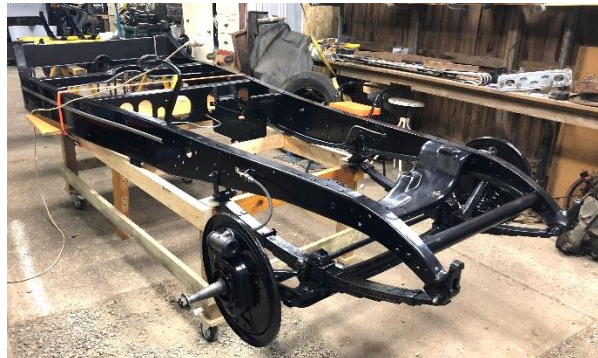
Chassis being re-assembled after painting
