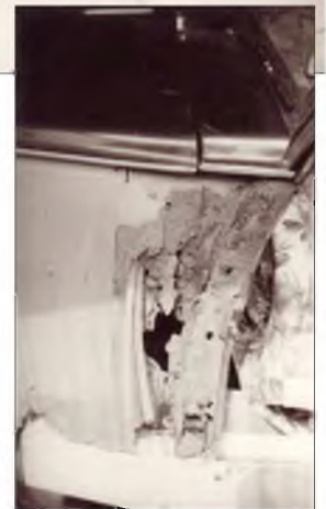
Main sill alongside the rusted old item.
