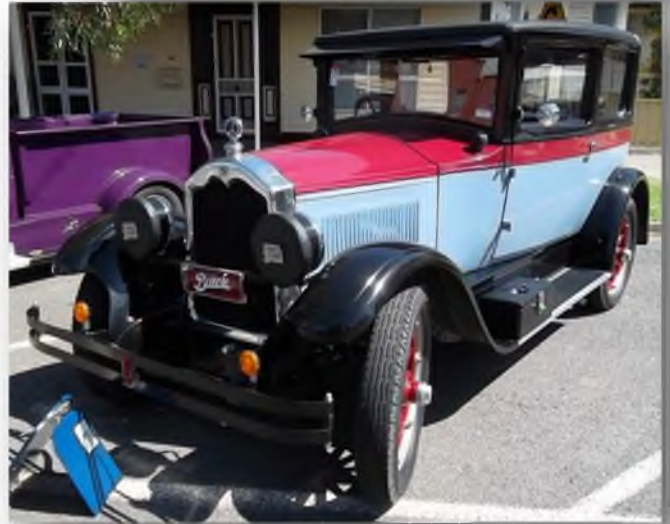
Model T Ford ute (top) (above) 1927 Buick 27-20X two door coach. Standard ohv 6 cyl, rated 23hp developed 63hp at 2800 rpm. Max stated speed 70mph. This is one of 870 exported from America to the world at a cost of $1,195US and weighed 3,215lb (1,481kg). 1927 sales slogan 'vibration beyond belief' Restored and owned by Alan & Lavinia Jolley.
