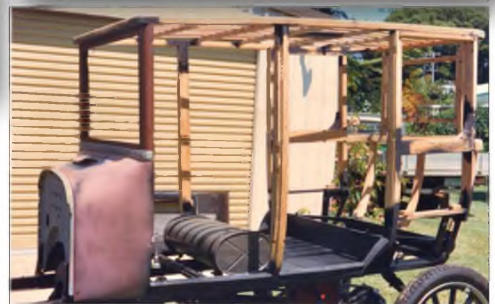
Having completed all the running gear the next task was to rebuild the body frame work. Stripping body panels from the frame work. Our Son Grant helped.
