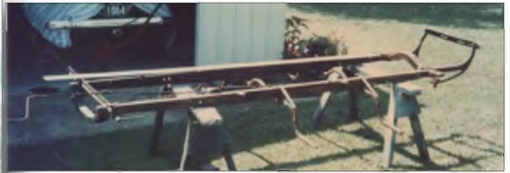
Straightening replacement chassis with chain and jack
