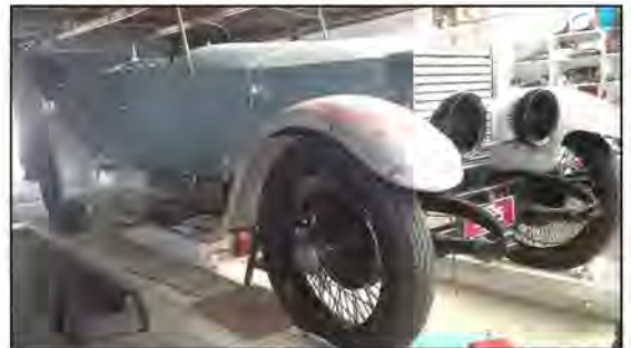
New valance panel and repairs being undertaken by Steve Barnett's workshop at Harcourt, not the correct 23 inch wheels
