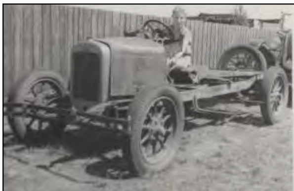
A 12/4 chassis was purchased for £15. We replaced the seized engine in the tourer with the engine from the chassis and hoped for the best
