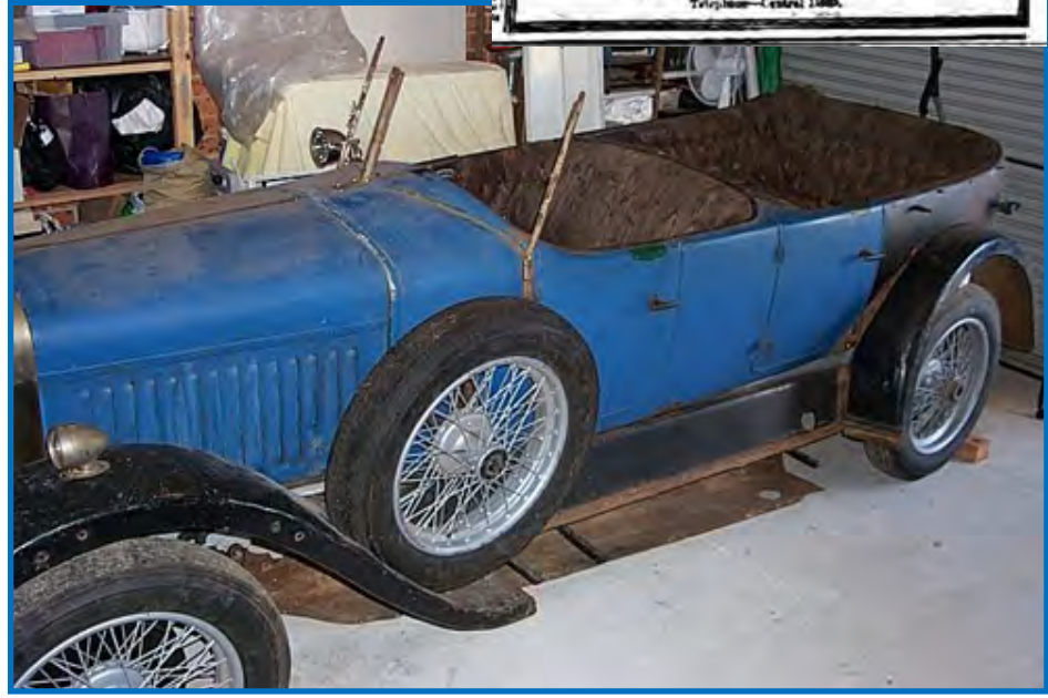
As it is today, complete but unrestored. Original upholstery is diamond pattern leather, which was probably a little old fashioned by 1922. You may just be able to pick up the timber capping. I assume my car was built to their standard design, but Burlington also built bodies to customer's designs.
