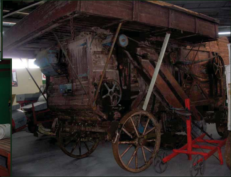
Clayton & Shuttleworth Thrasher built in Lincoln, England about 1890. It was driven by steam or stationery engine. Sheaves were tossed from a stack or wagon on top of the thrasher where two men would cut the binding. The stalks were then fed into the machine which separated and cleaned the grain. Straw would come out one end and several grades of grain would come out the other end. At least 6 men. And up to 10, were needed to operate the thrasher. This machine was used in the Kyneton, Trentham and Stuart Mill area until the 1930s
