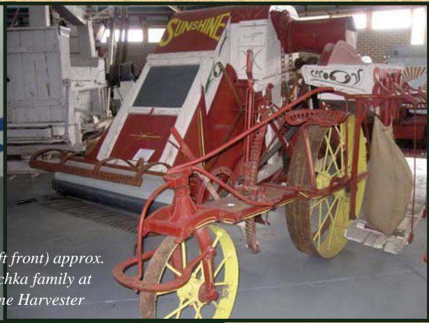
Clayton & Shuttleworth Thrasher built in Lincoln, England about 1890. It was driven by steam or stationery engine. Sheaves were tossed from a stack or wagon on top of the thrasher where two men would cut the binding. The stalks were then fed into the machine which separated and cleaned the grain. Straw would come out one end and several grades of grain would come out the other end. At least 6 men. And up to 10, were needed to operate the thrasher. This machine was used in the Kyneton, Trentham and Stuart Mill area until the 1930s
