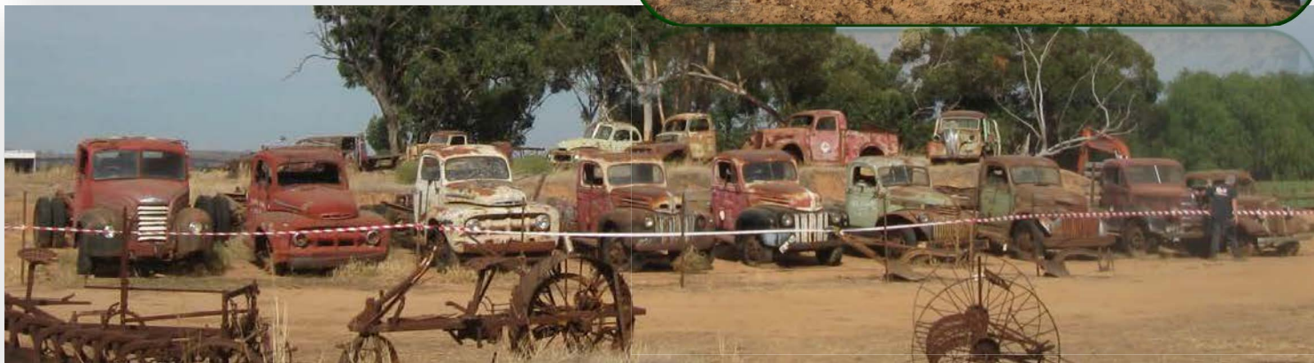
These are his older trucks plucked from local farms, many having sign writing on the doors with the farmer's name and town. A Ford Thames Trader V8, 2 early 1950's Ford V8s, 2 late forties Ford 'jail bar' V8s, 2 war time Chevrolets, a Bedford and half a 1934 Chevrolet. Like many trucks the back half was cut off to make a farm trailer. On the hill is an International, Ford V8, Commer utility (based on the Hillman Minx) and a Standard 10 saloon
