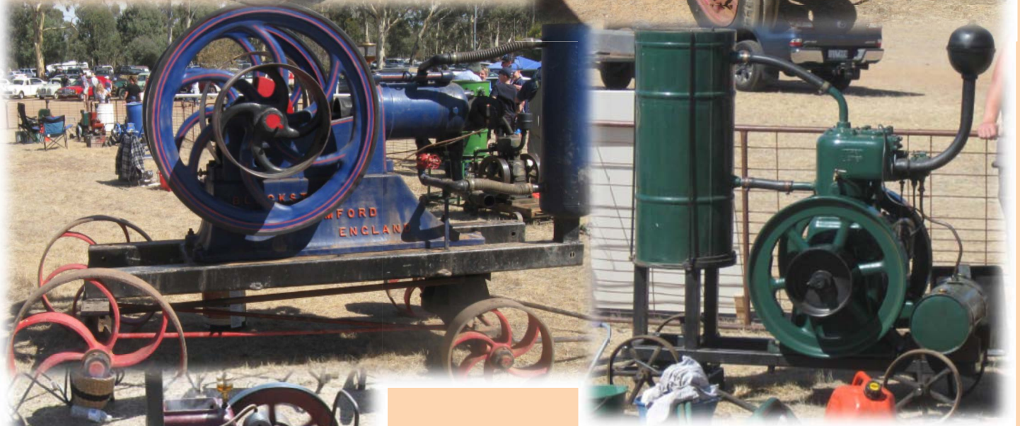
Vintage Tractor Pull, Lance Bulldog making a valiant attempt Pair of unrestored Lance Bulldogs David Brown tractor 1910 Blackstone 6½ hp oil engine, speed 250-300rpm. The engine spent a large part of its life providing the active power for a Mines Department of Victoria battery at Smiths Gully until it was retired due to the battery having been burnt down in the early 1960s. Lister vertical petrol engine 4hp built in 1918 owned by Rod & Jenny Medlyn of Stuart Mill. Sundial 2hp engine B type. It was used at the Nine Mile farm of Clive Olive for usual farm duties. Made in Sunshine by HV McKay. Owned & restored by Trevor Bailey & family, Wedderburn
